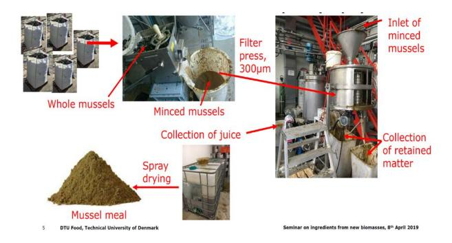
Results showed, that it was possible to produce a mussel meal product by this methodology, but that the product also had a relatively high content of ash (shell remains) despite sieving of the retained grinded juice.
