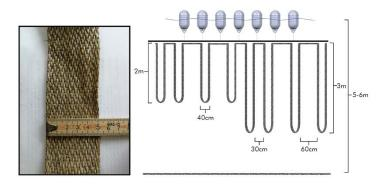
Figure 3: Experimental configuration of collector band spacing
